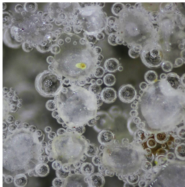
Proppant coated with AirRide treatment attracts the gas phase, which provides maximum suspension during operations.
